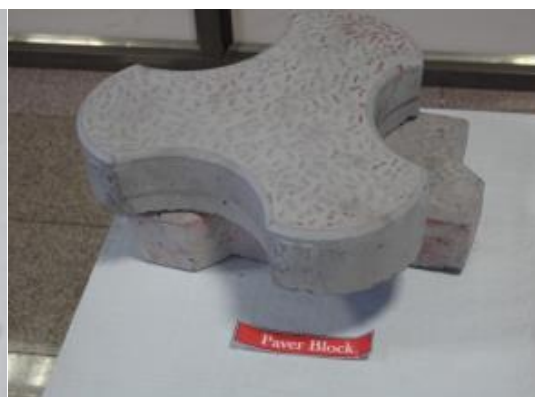
2. Paver Blocks made from Ground Granulated BF slag
