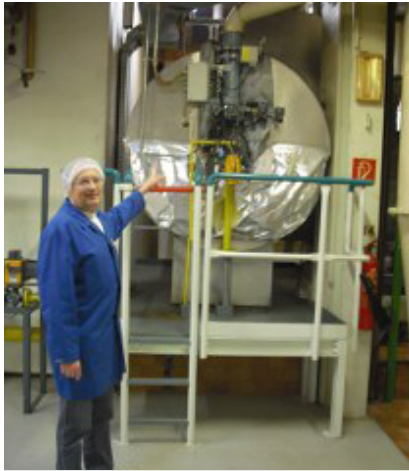
Helmut Plath in front of the RFB4 roaster's auxiliary burner, which ensures that the roasting machine's catalytic converter reaches its operating
