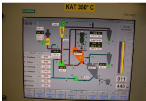
Each roaster has a screen which displays the exact status of the roasting process for each individual batch. The picture shows the screen of a RFB roaster running in test mode with an ultra low temperature catalytic converter.
